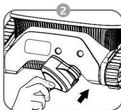
2 Connect the inductive charger to the robot
