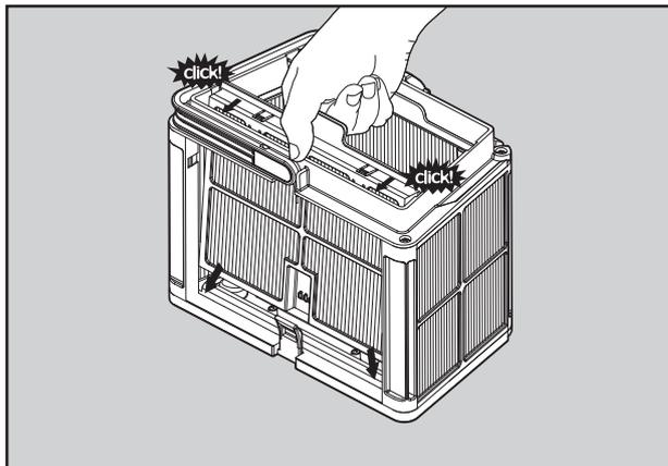
Re-assemble the filter panels.
