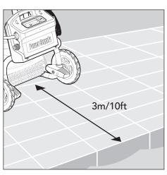
Position the power supply so that it is approximately in the middle of the long side of the pool at a distance of 3m/10ft.
