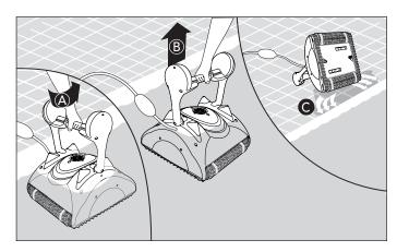
Place the Pool Cleaner on the edge of the pool and let the water drain out.
