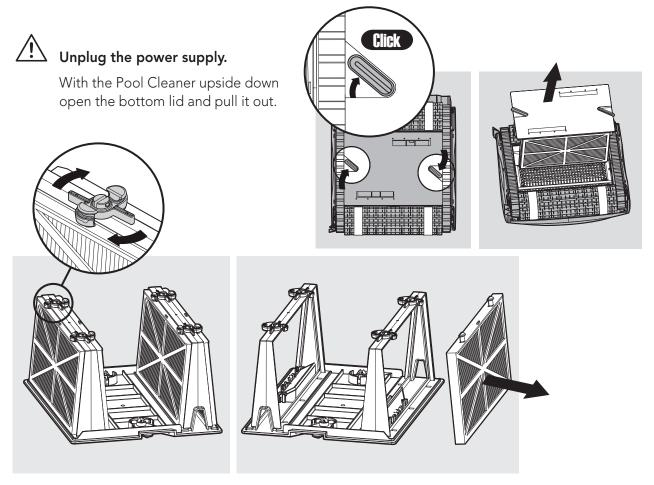
Open the clips and remove the filter.
